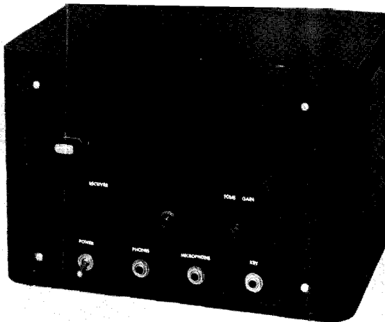
Figure 34 "DUPLEX" TRANSMITTER-RECEIVER FOR 220 MC. RADIO LINK
