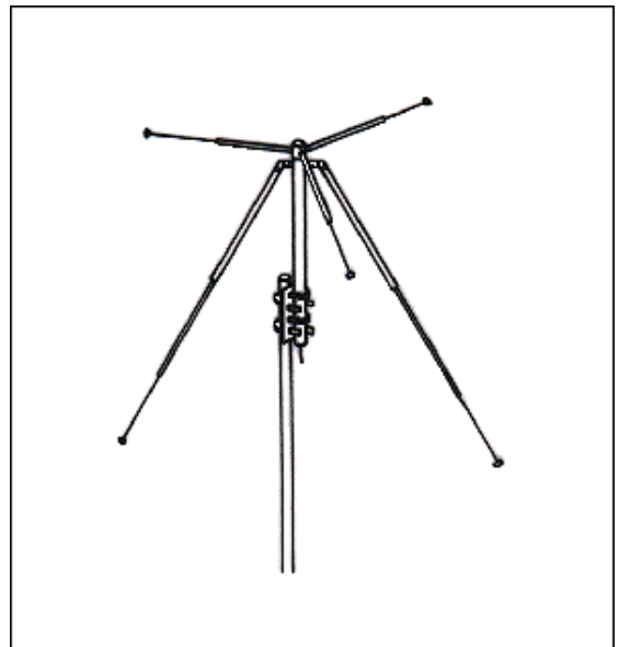
Figure 10.13 Mounting the completed antenna to the mast.
