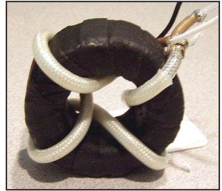
Fig 11-94 —9:1 transformer made by John, K9DX. The transformer has four trifilar turns. The trifilar wiring is made by using a small Teflon coax equipped with a second shield. See text for details.
