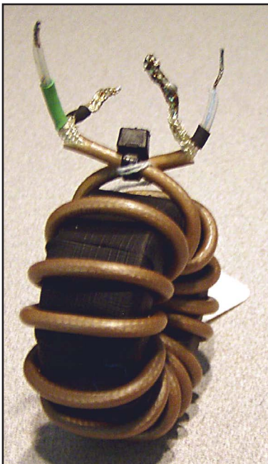
Fig 11-93 —K9DX made a 180^\circ 1:1 phase-reversal transformer wound using 13 turns of RG-303 coax on a two side-by-side, 2-inch OD #61 cores.
