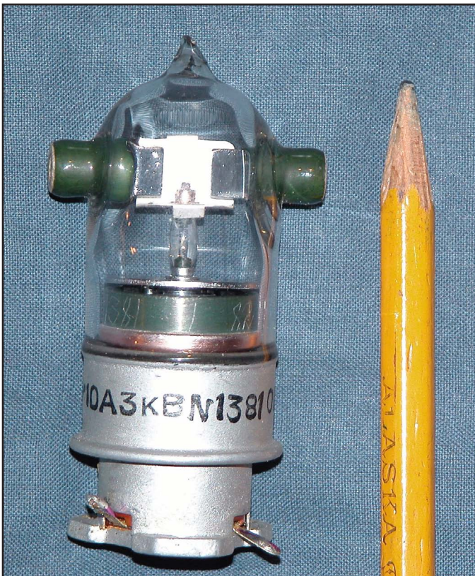
Fig 11-73—Russian-made small vacuum relays having single make/break contacts. These are well-suited for a relay matrix.
