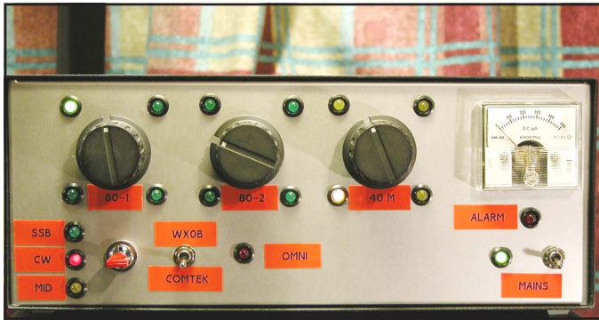
Fig 11-105—Array-direction switch box at ON4UN, with 1 direction switch for 40; 2 for 80. A switch selects the Comtek or Lahlum/WXØB system. Relative power and alarm circuit (Fig 11-104) is for Comtek. A lever switch selects one of three band segments on 80.
